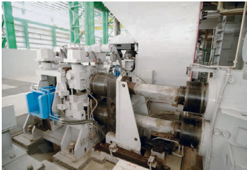
Red Ring stand with gear spindles
