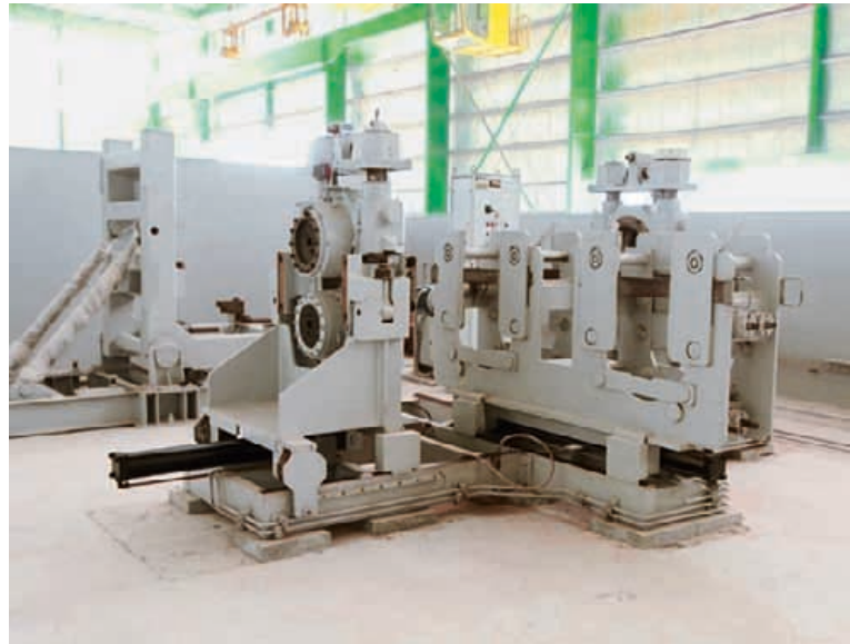
Hydraulic robot device for roll change
