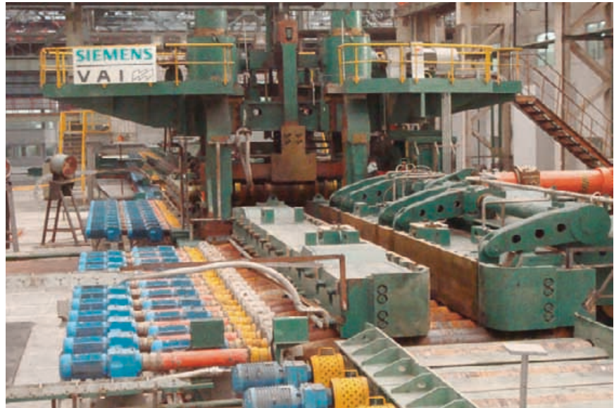
Sliding reversible 2-high stand with roller table and bar manipulator
